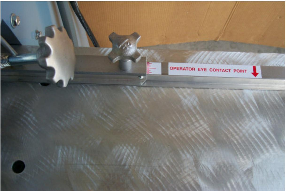
**Figure #2 Overhead View Fence Alignment Mechanism**
