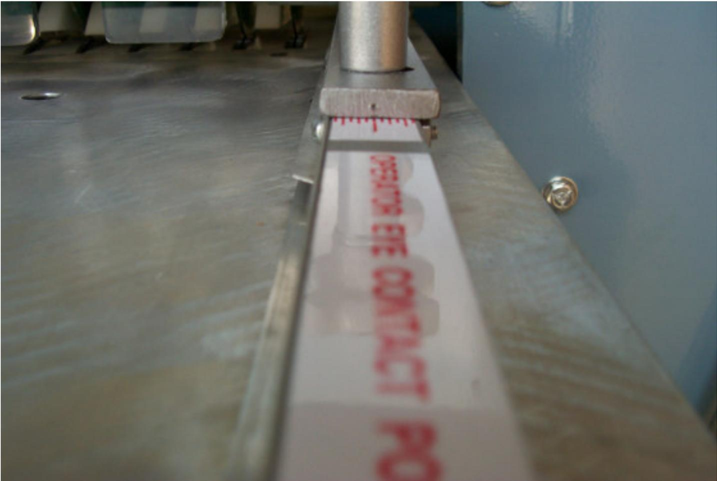
**Figure #1 Fence alignment mechanism punchmark and decal**
